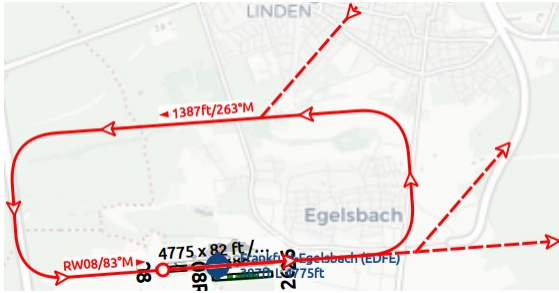
Traffic Pattern for the settings in the dialog above. Downwind leg shows pattern altitude above MSL and course and final leg shows runway name and course. White filled circle is the hotspot that can be right clicked to remove the pattern in the context menu. Click image to enlarge.
