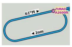
A hold with 2 NM straight segment length. Enter and exit at zunad and fly at or above 2,600 ft. Course is  $61^{\circ}$  magnetic degrees.
