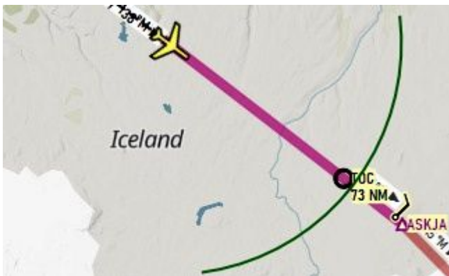
A jet aircraft climbing and about to reach the top of climb before waypoint ASKJA.
