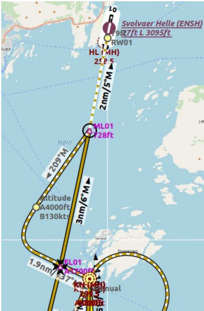
Straight In example: ENSH approach LOC FL01 (L01) to runway 01. White/orange dotted line is the straight-in leg. ML01 is the MAP. If runway is not visible at ML01 turn left to missed.
