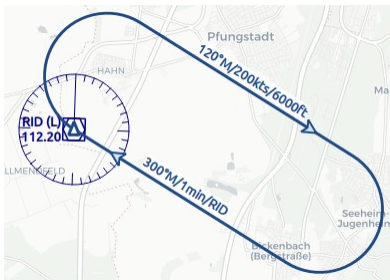
Holding at VORDME RID. Inbound label shows inbound magnetic course, holding time and navaid ident. Outbound track has outbound magnetic course, speed and altitude as label. While filled triangle is the hotspot and holding fix. Click image to enlarge.
