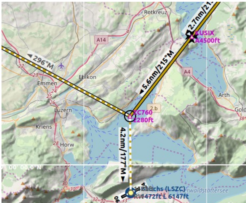
Circle to Land in example: LSZC RNAV-A KUSIX (RNAV). White/orange dotted line is the circle-to-land leg. ZC701 is the MAP. No guidance is given for this leg. You have to navigate around the mountain to get to runways 06 or 24.
