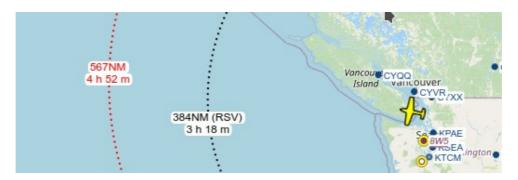
Aircraft endurance rings shown with labels. 384 NM and 3 hours and 18 minutes to go until on reserves as defined in aircraft performance. 587 NM and 4 hours and 52 minutes to go until fuel level is zero.
