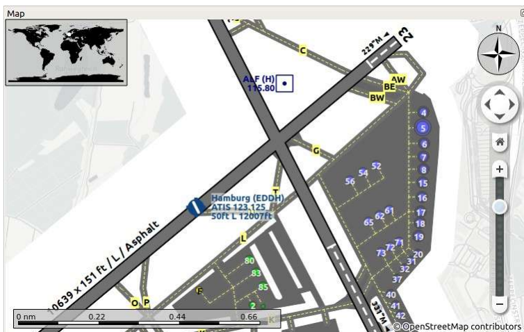
Detailed view of the airport diagram. Shows blue gates on the right and green general aviation ramp parking spots on the left. Long displaced threshold of runway 33 is visible. Dashed yellow lines indicate taxi paths. Click image to enlarge.
