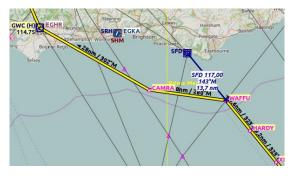
The same can be used when flying airways without GPS. In the example below fly 323 degrees magnetic to VOR SFD (radial 143). You are at WAFFU when the DME shows 13.7 NM. Then turn left to 280°M until you intercept 302° to GWC. *Click image to enlarge.*
