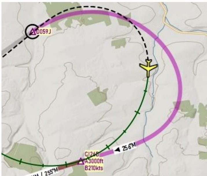
An aircraft turning in a procedure about to intercept the ILS after waypoint CI26B
