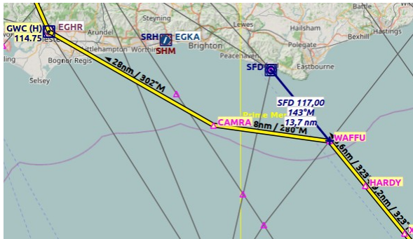
The same can be used when flying airways without GPS. In the example below fly 323 degrees magnetic to VOR SFD (radial 143). You are at WAFU when the DME shows 13.7 NM. Then turn left to 280°M until you intercept 302° to GWC. Click image to enlarge.
