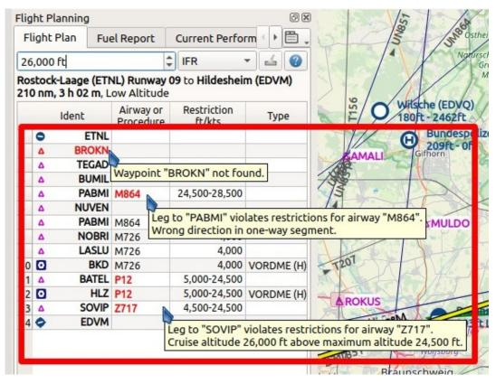
The Flight Planning with three different tooltips showing errors.
