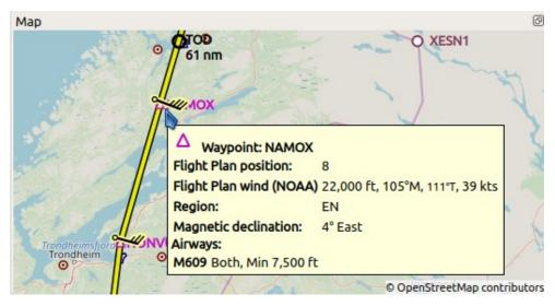
Wind barbs shown at flight plan waypoints and wind data in tooltip.
