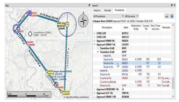
Showing a transition and a RNAV approach. Start and endpoint of a transition leg are highlighted on the map. Screenshot based on *Little Navmap* 2.6. *Click image to enlarge.*
