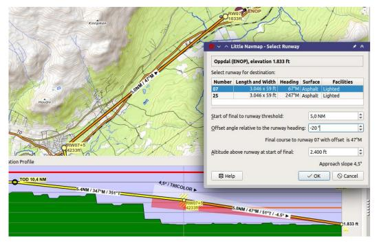
Destination runway dialog window and depiction on map and in elevation profile. Using 4.5° slope to match VASI and offset approach to avoid mountains. Vertical guidance to runway threshold. Note that ILS and other approach aids are not shown for the VFR approach. *Click image to enlarge*.
