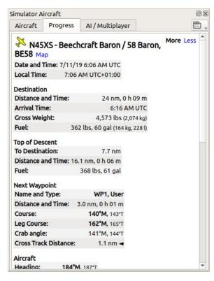
Aircraft progress information when connected to a flight simulator and user aircraft airborne. Alternate weight and fuel units (kg and liter) are enabled as well as true course display. *Click image to enlarge*.
