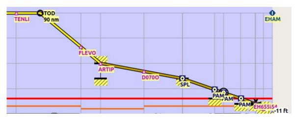
An approach procedure which requires the aircraft to descent early due to a restriction between 7,000 and 10,000 ft at ARTIP.
