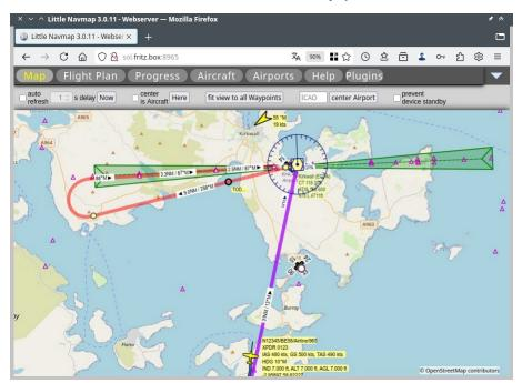
The map display in the *Little Navmap* web interface showing the flight plan, an approach procedure and the user aircraft. *Click image to enlarge*.
