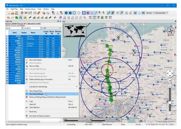
Radio navaid range rings along a flight plan. Click image to enlarge.
