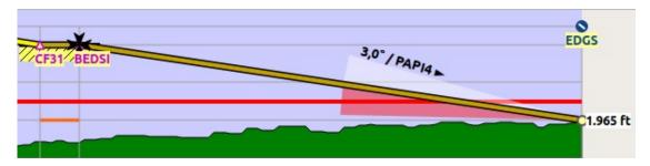
Display of VASI slope at destination airport. Slope is 3 degrees and VASI type is PAPI4. Final approach fix is marked with a Maltese cross.
