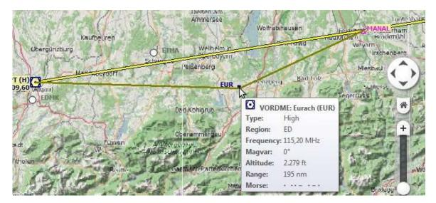
Inserting a navaid into a flight plan leg by clicking and moving the leg line. A tool tip for the navaid is shown.
