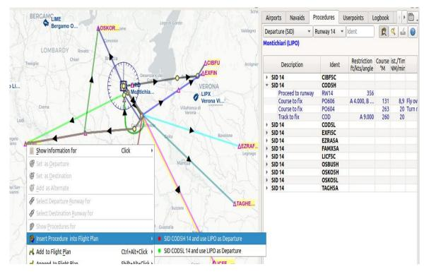
Previewing all SID at LIPO from runway 14. Context menu open to add SID and airport as departures. The preview also uses the Transparent line setting for flight plans in the options dialog on page Map Flight Plan. Click image to enlarge.
