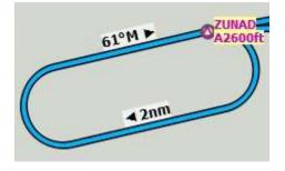
A hold with 2 NM straight segment length. Enter and exit at ZUNAD and fly at or above 2,600 ft. Course is 61° magnetic degrees.
