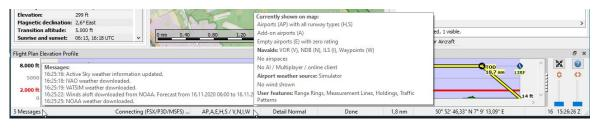
Status bar with messages in tooltip about the last weather updates, the connection status Connecting (FSX/P3D/MSFS) and a tooltip that indicates what is currently shown on the map. The map detail level is unchanged and the map coordinates at the cursor position are shown on the bottom right. Altitude at cursor is not shown since offline elevation data is not installed. The online map download progress indicator shows Done indicating all map tiles were downloaded. Zoom distance is 1.8 NM.
